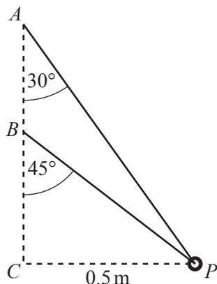
A small smooth ring  $P$  of mass  $0.4\text{ kg}$  is threaded onto a light inextensible string fixed at  $A$  and  $B$  as shown in the diagram, with  $A$  vertically above  $B$ . The string is inclined to the vertical at angles of  $30^\circ$  and  $45^\circ$  at  $A$  and  $B$  respectively.  $P$  moves in a horizontal circle of radius  $0.5\text{ m}$  about a point  $C$  vertically below  $B$ .
