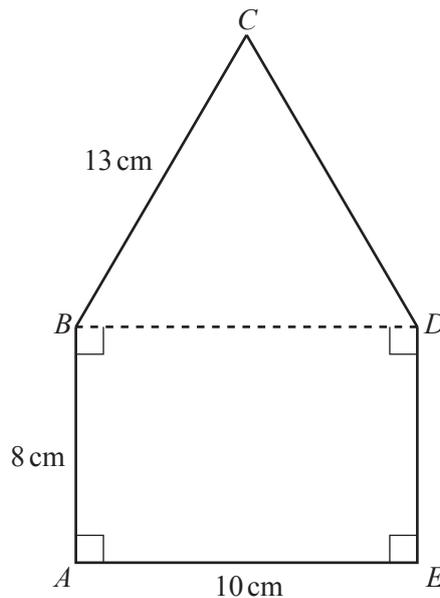
A uniform lamina  $ABCDE$  consists of a rectangle  $ABDE$  and an isosceles triangle  $BCD$  joined along their common edge.  $AB = DE = 8 \text{ cm}$ ,  $AE = BD = 10 \text{ cm}$  and  $BC = CD = 13 \text{ cm}$  (see diagram).
